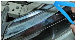
2.Measure the size and tear off the adhesive film
