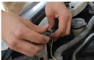
4. Take out turning bulb, yellow wire connect to turn signal socket positive power supply
