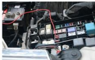
2. Red wire connect to ACC+ or headlight+
