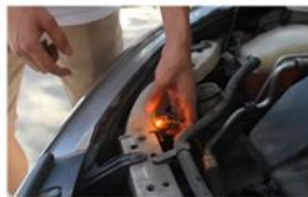
5. Install turning bulb back to the socket.
