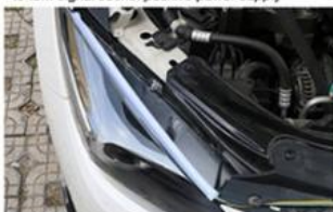
4. Take out turning bulb, yellow wire connect to turn signal socket positive power supply
